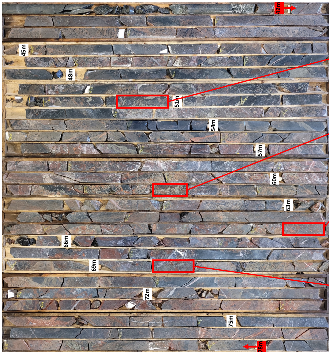
Figure 3. Dorland drill hole DP-23-06 sulphide breccia zone from 42 to 78 metres
